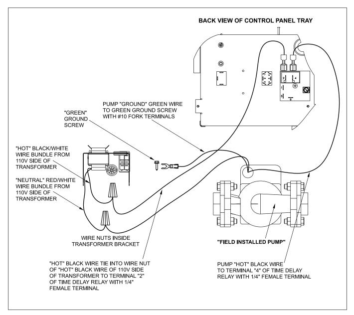
Figure 14. Field Wiring.
